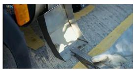
Disconnect the earth wire and place this back on the holder and replace the cover caps over the vent and filling connectors.
