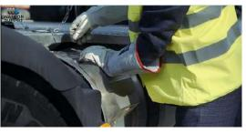
Close your tank cover. If the tank cover is not closed properly the vehicle micro-switch won't let the vehicle start, this is to prevent anyone driving off with any hoses still attached.
