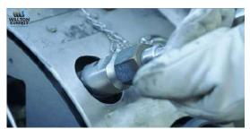
Connect the vent hose to your tank and then remove the filling nozzle from its holder.
