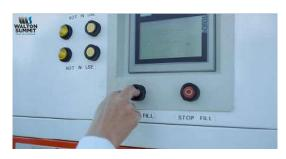
Go back to the main control panel and it will ask you to start filling, press the green start fill button and the filling process will begin.
