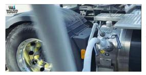
Once the filling has finished the first thing to be disconnected is the filling nozzle which can be released by pulling back the handles.
