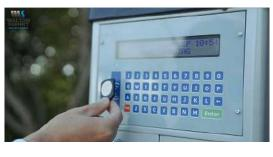
Then go to the authorisation machine, scan your filling tag and enter the information required (Registration and odometer reading).
