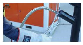
Remove the earth connection from the filling stand and connect this to the bottom of the tank cover (This must be present at all times).
