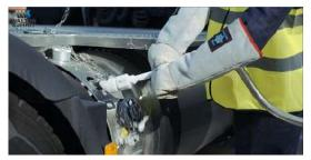
Then remove the vent hose by turning it anti-clockwise and place it back in its holder under the filling hose.
