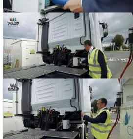
Hang the nozzle back on the pump and return to your vehicle. Replace the rubber bung in the connector box and close the door.
