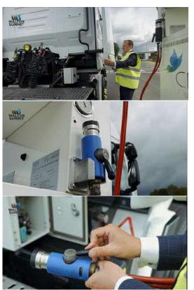
Move the air deflector out of your way to reveal a small box. Open the box door and remove the black rubber bung off the connector.
